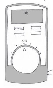
How much do the electrons you are providing want to get through your material? Higher voltage = greater "pushing force" through your wire, measured in volts.
