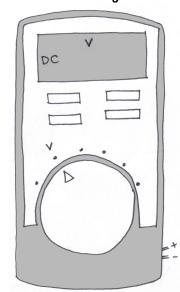
Is there a conductive path where electrons can flow? Test for faulty connections or short circuits.
