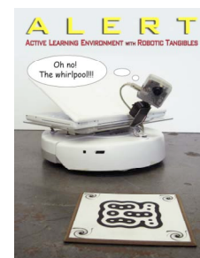
Figure 1: iRobot Create, laptop, and servo-mounted camera, observing a fiducial marker with human-legible whirlpool icons.
